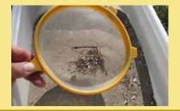
Smaller materials fall through the holes in the sieve, separating them from the larger particles which are left behind.
